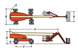
**Standard Features** Platform: 36 x 96 in. (0.91 x 2.44 m) Side Entry 8 ft (2.44 m) JibPLUS® Boom Selectable Capacity Envelope 180° Hydraulic Platform Rotator AC Receptacle in the Platform 5 Degree Tilt Alarm/Indicator Light All Motion Alarm Swing-Out Engine Tray 12V DC Auxiliary Power Hourmeter Control ADE° System Full-time 4WD 3 Selectable Steering Modes Drive-out Extendible Axles
